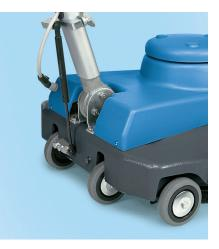
The gas shock helps maintain constant brush pressure on the floor, regardless of the position of the steering column.
